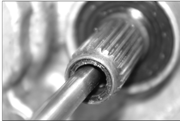
Worn bushing in clutch pushrod.
